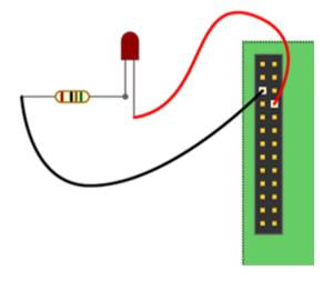
echo 0 > /sys/class/gpio/gpio11/value
