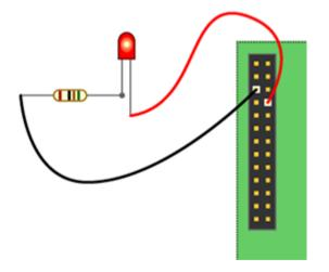
echo 1 > /sys/class/gpio/gpio11/value
